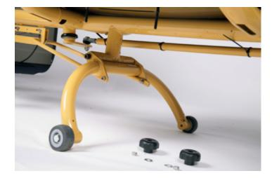
When the desired position of the seats is Chosen they can be attached to the floor board. First slide the threadpint throught the pod and floorboard in the right position.
