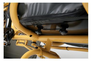
Screw on the wingnuts and tighten them The locknuts are only installed to make sure the wingnuts cannot fall of, they do not need te bee tightened completely
