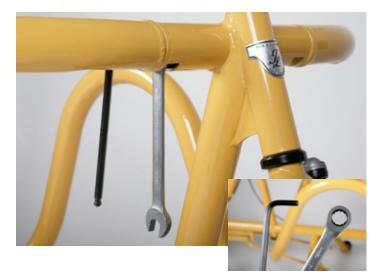
Check alignment and adjust if necessary Tighten the bolts using the ratchet ring spanner.
