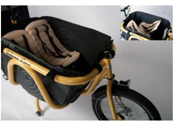
The seats can be positioned forward and backward and are able to slide backwards and forwards. When the seat are positioned opposite of each other, one facing forward and one facing backward, the shoulders of the children will not be aligned and there will be more room for taller children
