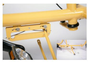
With the center tube in place, the positioning rod can be connected.
