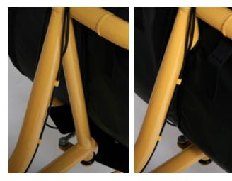
Form the soft pod around the steering tube.
