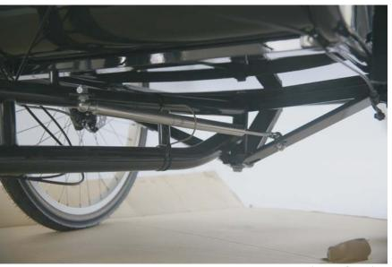
Connect the steering damper to frame and triangle as shown in picture. Check if the 'extending rod' side is mounted to the triangle.
