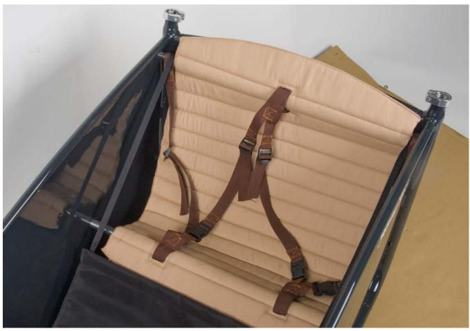
all parts of seat installed correctly
