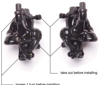
loosen 1 turn before installing (on both brake claws)
